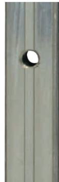
Rail with CZS coating – after 99 hours of salt spray test (acc. to DIN EN ISO 9227)
