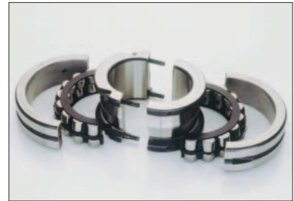
4: Split spherical roller bearing with split solid cage made from glass fibre reinforced polyamide or brass, with integral locking rings
