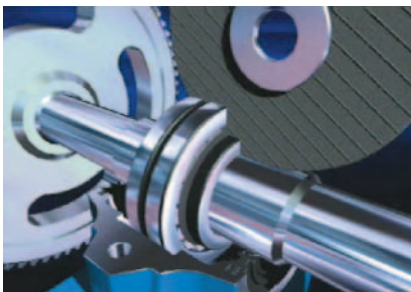
3 Dismount the old bearing (unsplit bearings with adapter sleeve should be carefully cut through using a parting-off grinder)
