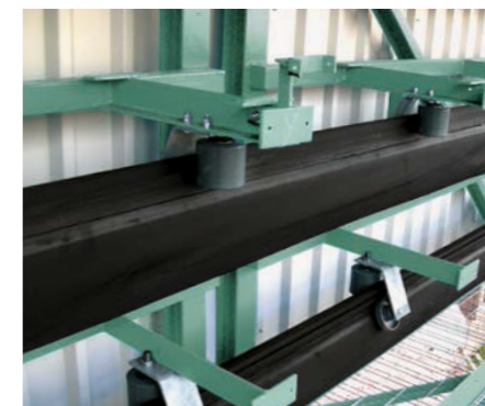
High-care transport thanks to enclosed belt design
