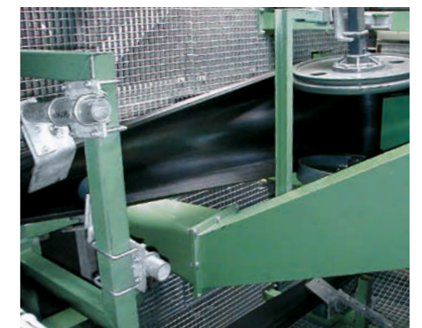
Does not pollute thanks to enclosed belt on return trip
