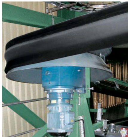
Good curve negotiability eliminates need for transfer points
