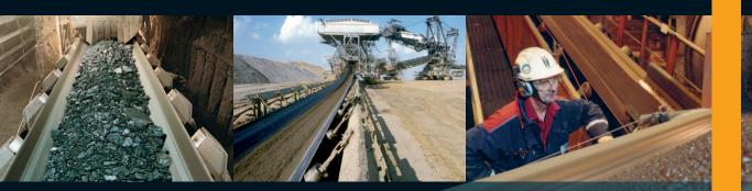
ContiTech has developed fabric and steel cord conveyor belts which meet the much higher requirements of EN 12882 and EN 14973. Due to our many years of experience in the field of fire safety, we are able to offer our customers conveyor belts certified by an external test institute.
