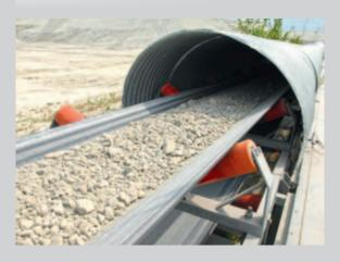
The crushed limestone is generally transported by means of conveyor belts which have to cover very long distances. STAHLCORD® conveyor belts are used here. Thanks to their structure, they can resist high impact energy and are easily troughable. Transverse reinforcement can be worked into the belt structure to improve impact resilience even further.
